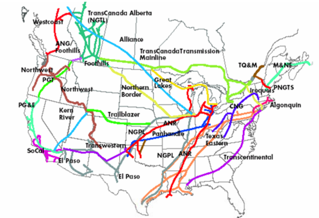
Figure 12.1: Canadian and US Natural Gas Pipelines
